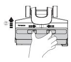
Squeeze latches on the cover and pull upward to remove.
