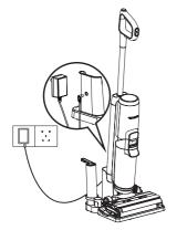
To charge the appliance, place the appliance on the charging dock and plug the adaptor into a power outlet.
