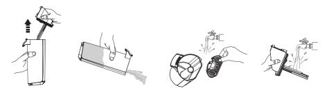
If the Dirty Water Tank lid and the filter inside have been blocked, remove the tank lid and the filter, rinse both parts with water.
