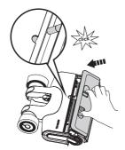
While replacing, always latch the brush cover into place to avoid leakage.
