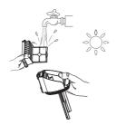
Grasp recessed area on each side of the dry filter and pull upward. Rinse under running water and must be completely dry before recombining with the lid of the DWT.
